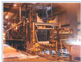
Indirect heating using radiant tubes for a continuous heat-treating furnace
