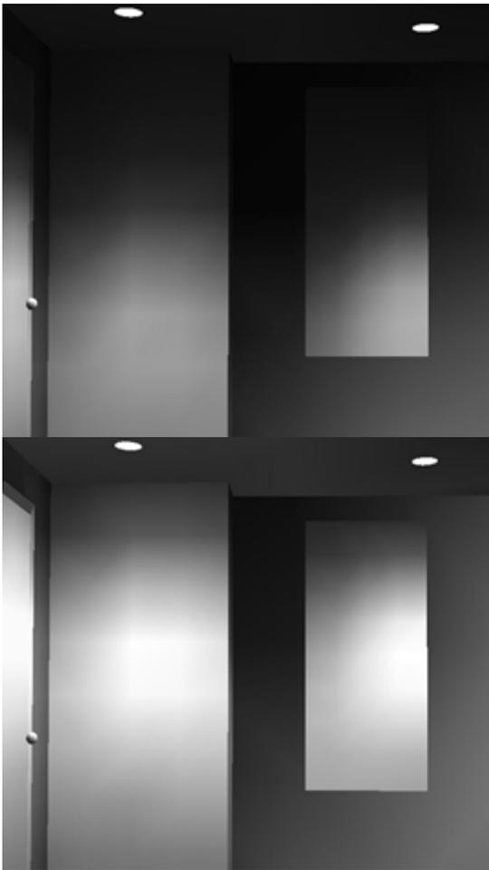
Grayscale renderings of the entry area, based on simulations of LED (bottom) vs. halogen PAR lamp (top) downlights. The PAR lamp downlight provided higher illuminances on the floor but produced dark walls. The LED downlight provided more light onto the walls, and also produced better lighting for visual tasks such as selecting clothing from the closet and evaluating appearance in the mirror.
