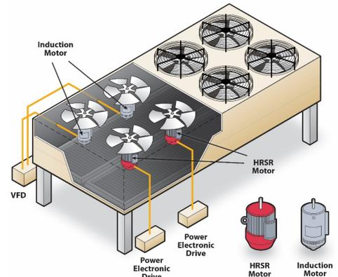
Figure 1: Installation of HRSR motors
