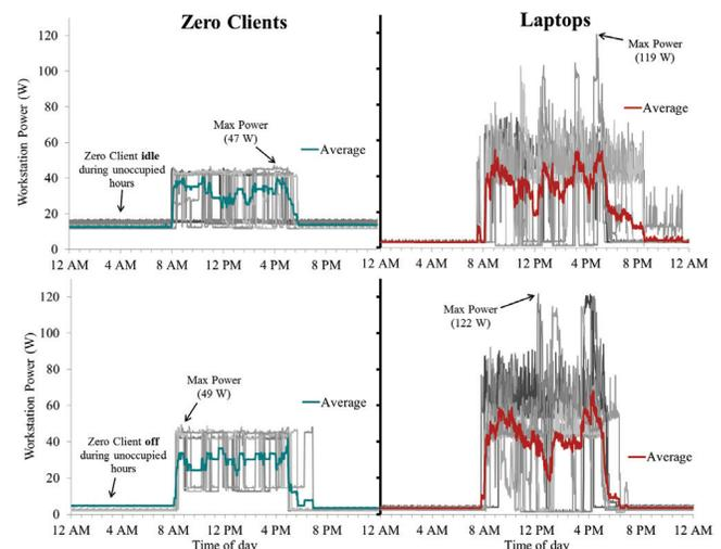
**Figure 1.** The electricity consumption of two zero-client workstations compared with two laptop workstations over a 2-week study. These graphs highlight the energy savings that can be achieved when workers are at their workstations.
