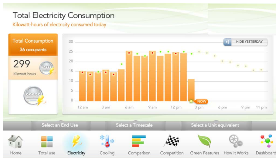
FIGURE 3: EXAMPLE EIS SCREENSHOT (LUCID), A BAR GRAPH TRACKING ENERGY CONSUMPTION PATTERN AT AN HOURLY INTERVAL
