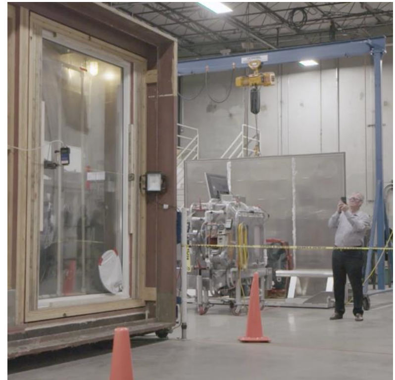
Pressure testing 50sf thin-glass triple pane
