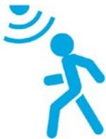
**Occupancy-based controls** – Occupancy sensors automatically turn on the lighting when motion is detected and automatically reduce or turn off the lighting when no occupancy is detected. Vacancy sensors are manually switched on and automatically turn off when no motion is detected.
