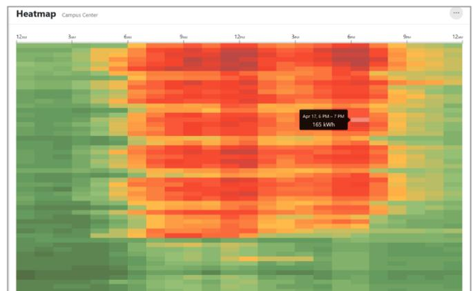
A 'heat map' provides visualization of energy use over a 24-hour period (horizontal axis) for many days (vertical axis). Red is high energy use; green is low energy use.
