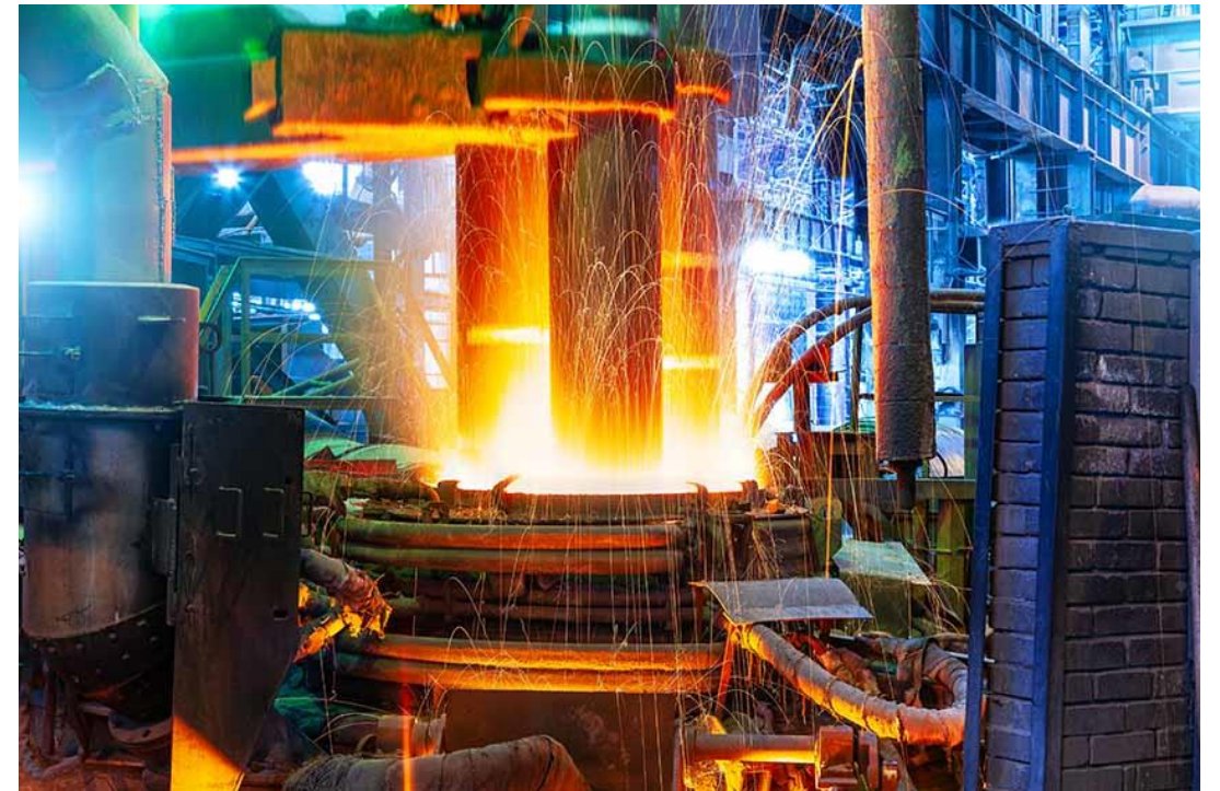
An electric arc furnace used in steel mini-mills
