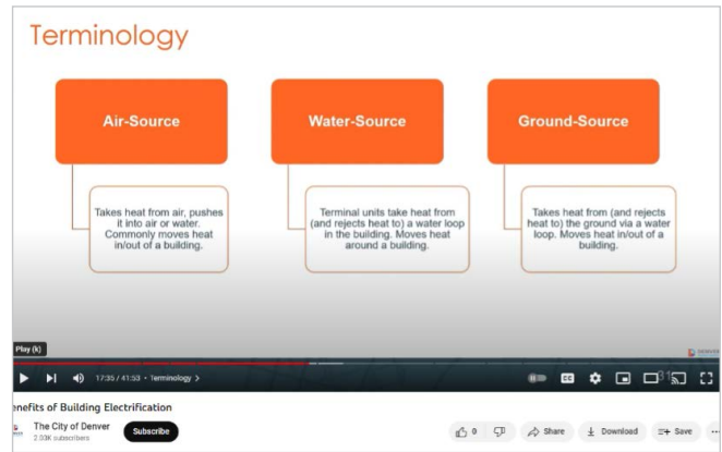
Screenshot from the Benefits of Building Electrification webinar defining relevant heat pump terminology
